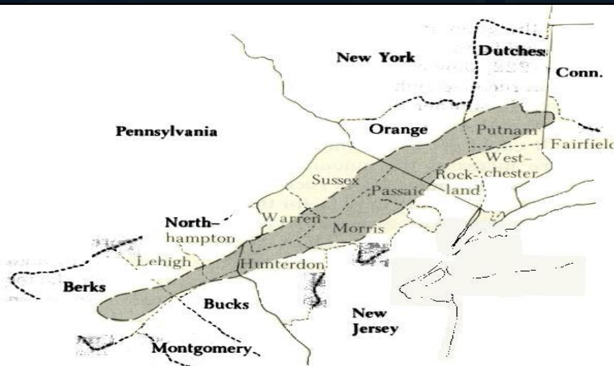
FIGURE 4-8 The shaded area indicates the extent of the so-called “Reading Prong.” This geologic region, consisting mostly of granite, contains a much higher-than-average number of houses with high indoor radon levels. (Reprinted with permission from R.L. Fleischer, Health Physics 50. Copyright 1986, Pergamon Press plc.)
